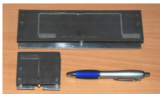
Fig 10: Hardware of PDA & Two elements CPDA with reflector
